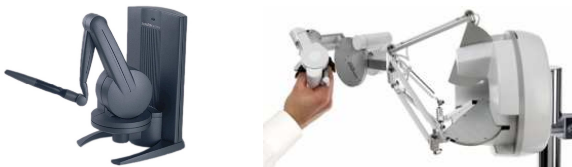
Rys. 7. Manipulator Geomagic Touch X (po lewej) [8] oraz Force Dimension Sigma 7 (po prawej) [9] Fig. 7. Manipulators: Geomagic Touch X (on the left) [8] and Force Dimension Sigma 7 (on the right) [9]
